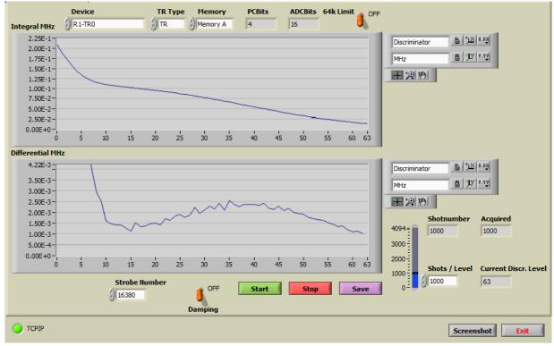
Please notice the change in the slope around discriminator level 10. The differential PHD for the same light intensity makes that more obvious. Select the differential field on the right side of the data display to get the differential PHD.
