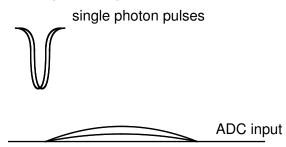
If two single pulses overlap the signal at the ADC will increase proportional. Due to this effect the ADC does not have a dead time constraint even for high count rates. For high count rates the linearity of the analog signal is superior to the photon counting.
